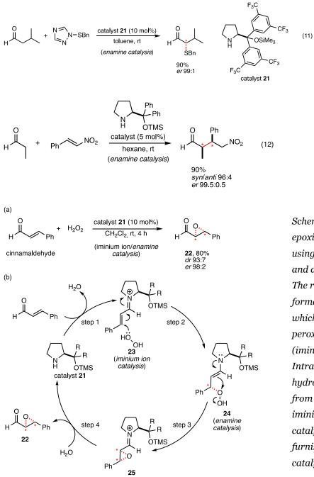
Scheme 3. (a) Organocatalytic epoxidation of cinnamaldehyde using hydrogen peroxide  $(H_2O_2)$ and diarylprolinol catalyst 21. (b) The reaction proceeds by initial formation of iminium ion **23**, which is attacked by hydrogen peroxide to form enamine 24 (iminium ion catalysis). Intramolecular expulsion of hydroxide ion, or its equivalent, from this species generates iminium ion 25 (enamine catalysis) which is hydrolysed to furnish epoxide **22** and regenerate catalyst 21.
