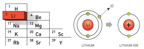
Lithium is a metal. It has just one electron in its outer electron shell, and this has a strong drive to leave lithium for another atom. When this happens, a positively charged – and more stable – lithium ion is formed.
