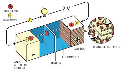
The first rechargeable batteries had solid materials in the electrodes, which broke down when they reacted chemically with the electrolyte. This destroyed the batteries. The advantage of Whittingham's lithium battery was that lithium ions were stored in spaces in the titanium disulphide in the cathode. When the battery was used, lithium ions flowed from the lithium in the anode to the titanium disulphide in the cathode. When the battery was charged, the lithium ions flowed back again.
