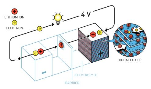
Goodenough started to use cobalt oxide in the lithium battery's cathode. This almost doubled the battery's potential and made it much more powerful.
