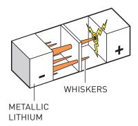
Whiskers of lithium form when a battery with pure lithium in the anode is charged. These can short-circuit the battery and cause fires and even explosions.
