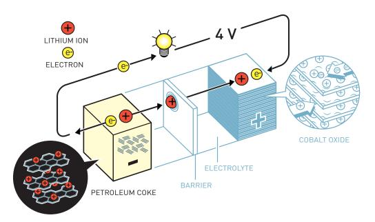
Akira Yoshino developed the first commercially viable lithium-ion battery. He used Goodenough's lithium-cobalt oxide in the cathode and in the anode he used a carbon material, petroleum coke, which can also intercalate lithium ions. The battery's functionality is not based upon any damaging chemical reactions. Instead, the lithium ions flow back and forth between the electrodes, which gives the battery a long life.
