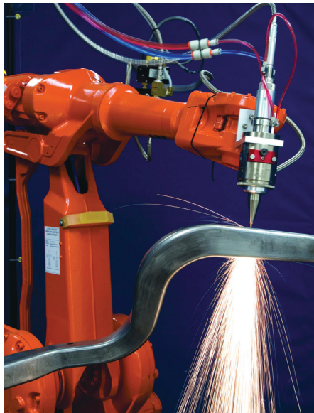
The fibre laser has become a valuable materials processing tool, with output powers reaching 10 kW for single-mode devices and 50 kW for multimode devices.
