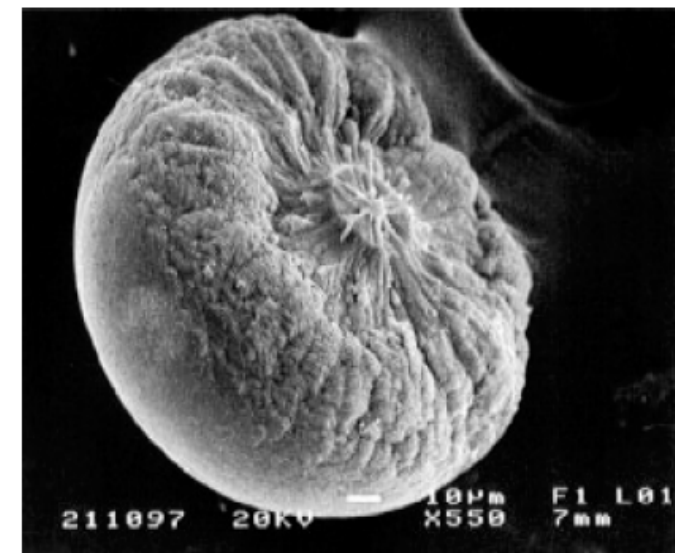
Fig. 4. SEM image showing half of an equatorially notched fluorapatite-gelatin spheroid. Scale bar is 10 \mu m. Reproduced with permission from Chemistry of Materials [30]. Copyright 2001 American Chemical Society.
