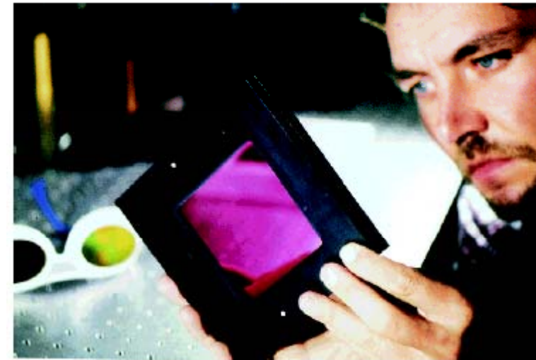
Figure 13. Bacteriorhodopsin film with large aperture. These films have free apertures of 90 mm × 90 mm, their outer dimensions are 120 mm × 120 mm. They are tuned to maximal light sensitivity because their primary use is in holographic interferometry.
