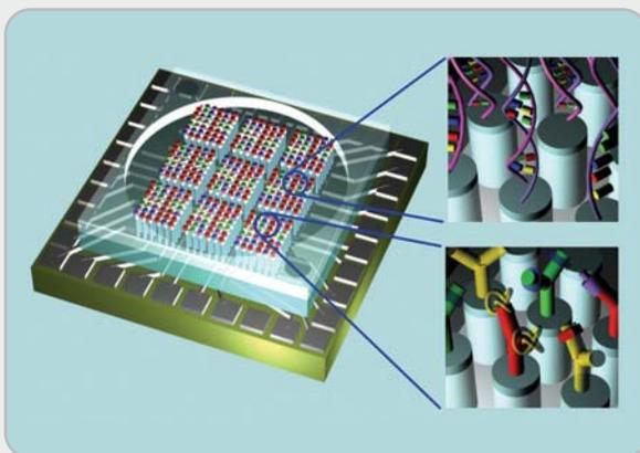
At left is an artist's conception of an ultrasensitive multiplex electronics biosensor based on a carbon nanotube nanoelectrode array. The insets on the right represent applications in DNA (top) and antigen detection (bottom).
