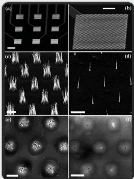
At left are scanning electron microscope (SEM) images of: (a) a 3x3 array of electrode pads, (b) an array of MWNT bundles on one of the electrode pads, (c, d) an array of MWNTs at UV lithography and e-beam patterned Ni spots, respectively, (e, f) the surface of polished MWNT array electrodes grown on 2-micrometer and 200-nanometer spots, respectively.
