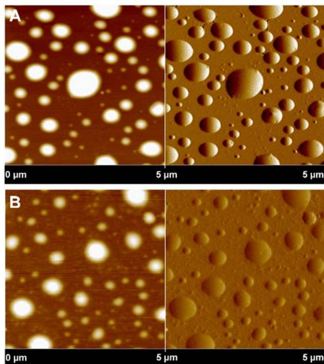
Fig. 2. Atomic force micrographs showing surface properties of polymer nanoparticles prepared from (A) PVA<sub>300</sub>-g-PLGA(15), and (B) fluorescence-labelled PVA<sub>300</sub>-g-PLGA(15). Each single image has an edge length of 5 μm.
