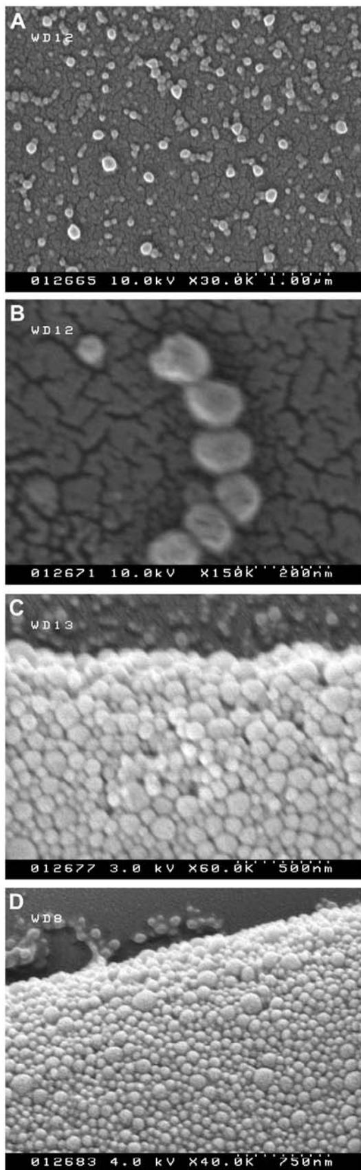
Fig. 1. Scanning electron micrographs of nanoparticles prepared from (A), (B) PVA<sub>300</sub>-g-PLGA(30), (C) PVA<sub>300</sub>-g-PLGA(15), and (D) fluorescence-labelled PVA<sub>300</sub>-g-PLGA(15) loaded with 0.5% paclitaxel in different magnifications.
