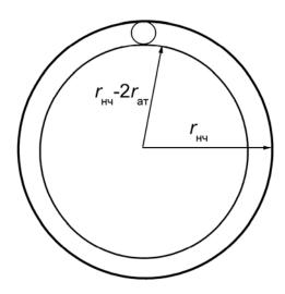
$$V_{\text{пов}} / V_{\text{HY}} = (4/3\pi r_{\text{HY}}^3 - 4/3\pi (r_{\text{HY}} - 2 r_{\text{aT}})^3) / 4/3\pi r_{\text{HY}}^3 = (r_{\text{HY}}^3 - (r_{\text{HY}} - 2 r_{\text{aT}})^3) / r_{\text{HY}}^3 = (1.5^3 - (1.5 - 2.0.144)^3) / 1.5^3 = 0.47 = 47\%$$
