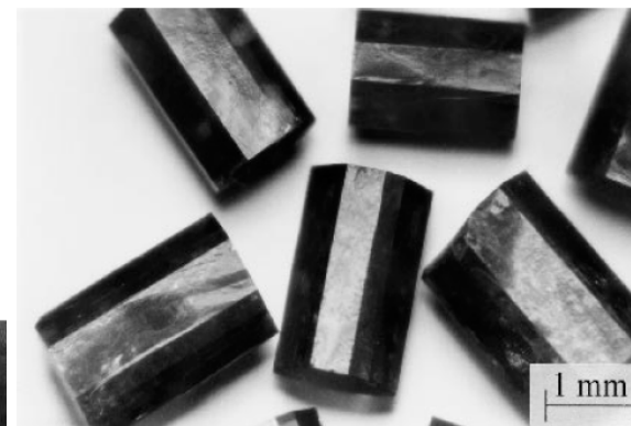
Fig. 17.9. Emerald crystals grown from \text{Li}_2\text{O}-\text{MoO}_3 flux
