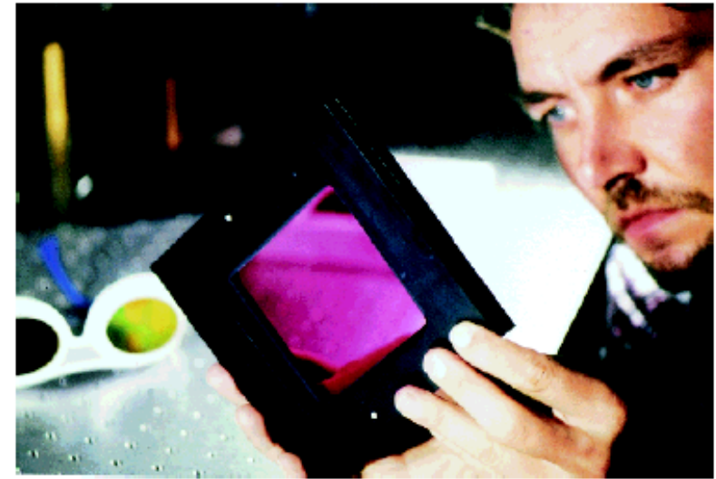
Figure 13. Bacteriorhodopsin film with large aperture. These films have free apertures of 90 mm × 90 mm, their outer dimensions are 120 mm × 120 mm. They are tuned to maximal light sensitivity because their primary use is in holographic interferometry.
