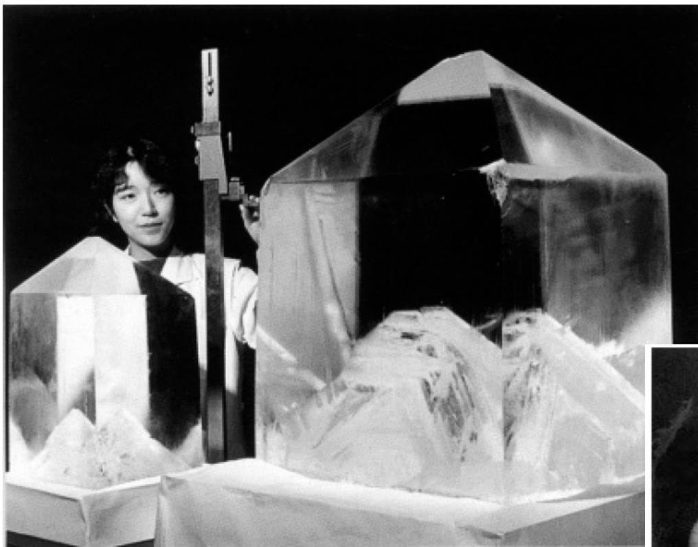
KDP crystals (size 45 \times 45 \times 70 \text{ cm}^3 , growth period one year).
