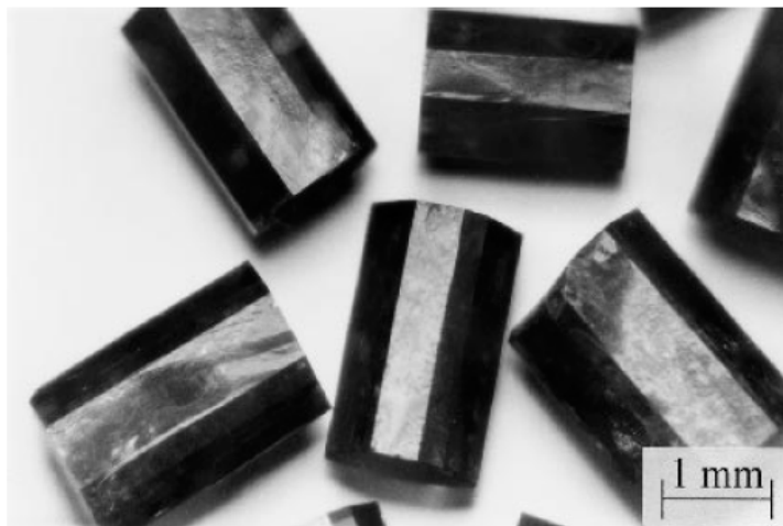
Fig. 17.9. Emerald crystals grown from \text{Li}_2\text{O-MoO}_3 flux
